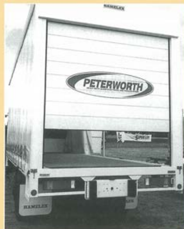
The Peterworth roller shutter door.
