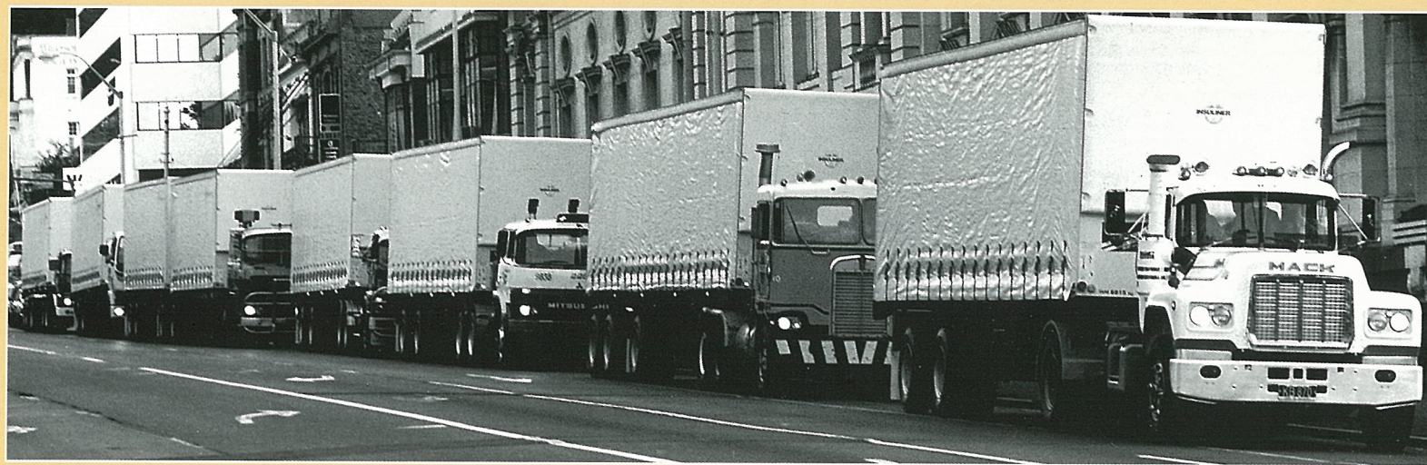
A convoy of the "sider" type of trailers that Neil Peterken introduced to NZ.
