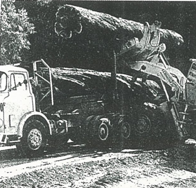
A 25-ton payload coming up for this spaced axle trailer, made by N.Z. Arc Welding Works Ltd. The trailer is being loaded with native timbers in the Kaingaroa State Forest.
